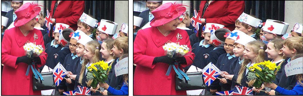
The picture on the left is a correctly-proportioned 4:3 image of a familiar figure. The image on the right shows the commonly-encountered effect when 16:9 equipment is unable to aspect-correct mixed image formats stretches them instead. Each person winds up looking too wide.
